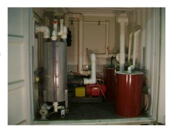
other stand alone equipment such as an electrically heated catalytic oxidizer.
